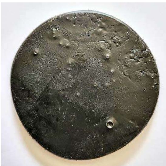
Lignik Composite Sample. Lignik products can be designed to be 3D-printed as a single unit or be utilized in wall panel-based constructions (Photo by A. Ghayur. 2019. Latrobe Valley circular industrial ecosystem. Federation University Australia. PhD dissertation: pp. 108)
